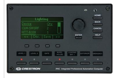
The IPAC-GL1 is designed to be mounted in a standard 3-gang electrical box independent of the lighting panels, allowing it to be installed wherever it is most advantageous for the project.
